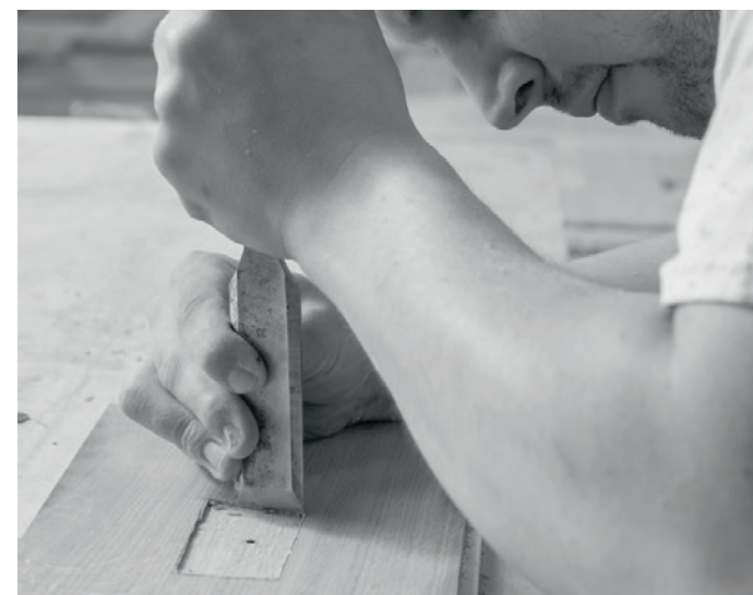
Applying the steel inserts.
